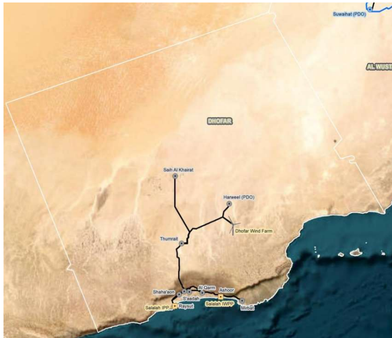
Figure 5.1-1 132 kV grid substations forming the regional transmission network in the Dhofar Region
